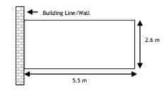
4. Perpendicular bays – a 0.8m overspill is required.
