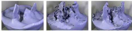
Fig2: An example of existing grid-based solution 10 . From left to right: simulated on coarse grids, after enhancement, simulated with fine grids. The enhanced fluid is not consistent to the fine grid simulation, which the ER will address.
